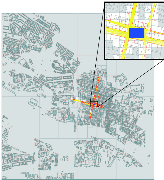
Fig. 1. Illustration of the from-region visibility in 2D. The scene represents a 2D footprint of 25\text{km}^2 of Glasgow city containing 94460 line segments. The PVS formed by the occluders visible from the given region is shown in red. The yellow lines depict visibility discontinuities.
