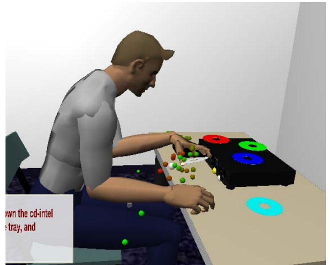
Figure 5: A screenshot of the activity reconstructed in VR. Small green and red spheres indicate the hand trajectory.
