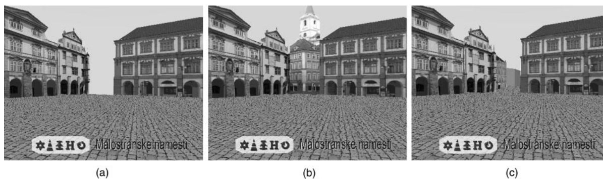
Figure 4. Impostors temporarily placed at sector gates improve the visual look. (a) An individual sector without any impostor. (b) Impostor at a gate. (c) A neighboring sector was loaded and the original impostor removed. The house in the background has no texture. This sequence of snapshots is a rather negative example, since the impostor was created using a photo taken from an inappropriate position. Big differences and even quality degradation can be seen when snapshots (b) and (c) are compared. Impostors should be made of images resulting from 3D models.
