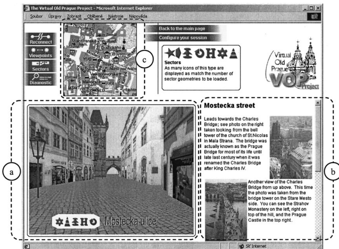
Figure 2. A web page with a virtual city can contain several interactive components allowing synchronized multimedia presentation. The example taken from the Virtual Old Prague project shows the three most important parts. (a) A 3D scene window. (b) An HTML document. (c) A 2D navigation map.
