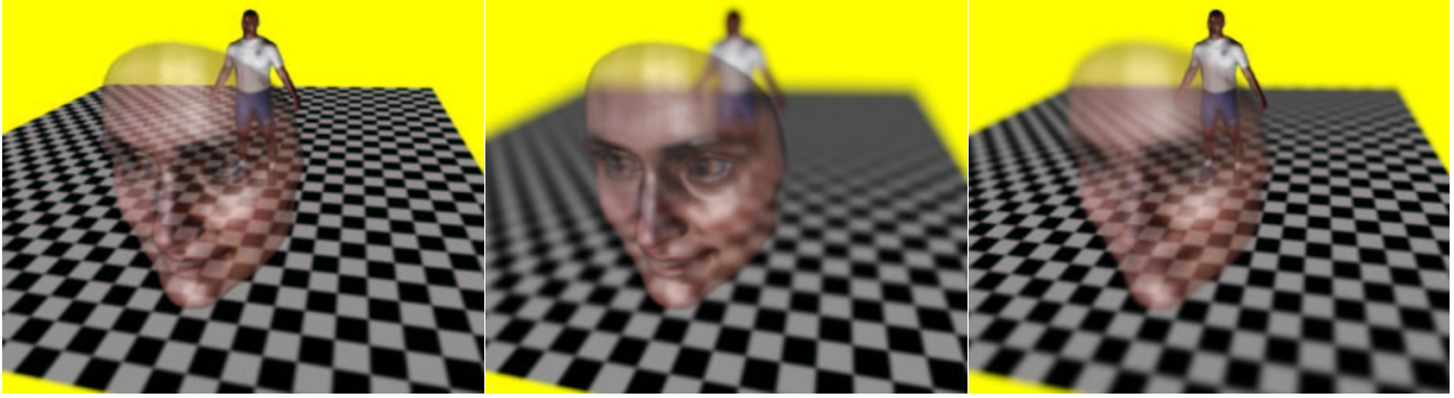
Figure 1. Example of DOF rendering with semitransparent surface. Left: no DOF. Middle: DOF is on and the transparent mask is in focus. Right: the male body is in focus, the mask is out of focus.
