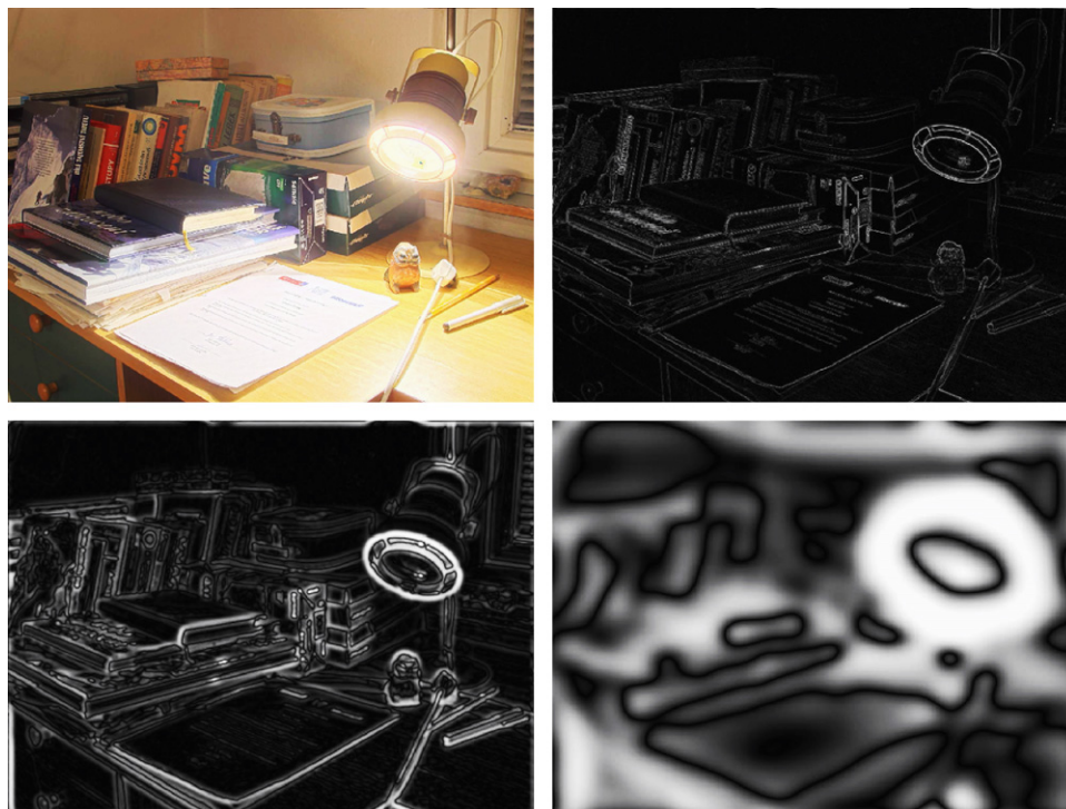
Fig. 1. Peli's local band-limited contrast on three different spatial resolutions (top-left: original image).
