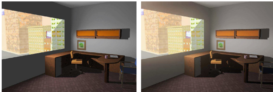
Fig. 5. Bloom (veiling luminance) simulation. Left: the original scene without bloom simulation. Right: the same scene with bloom simulation. Source HDR image courtesy of Greg Ward.
