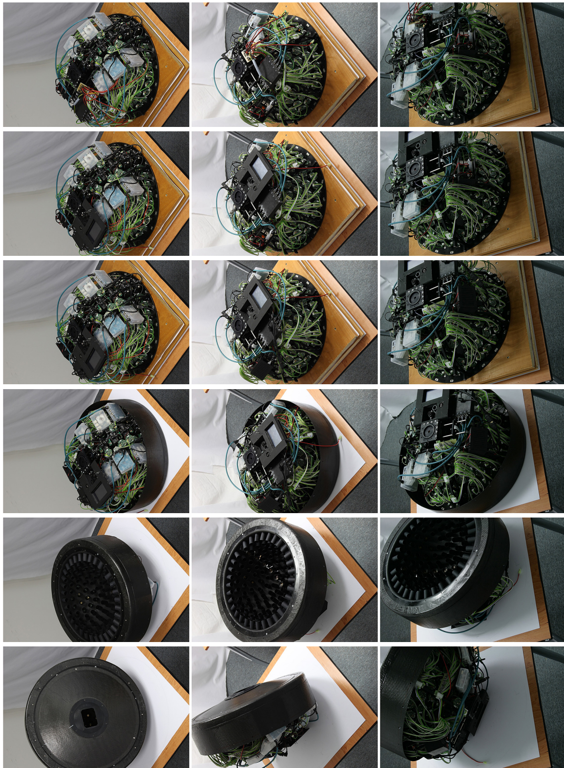
Figure A4. Assembly of lightdrum, step 19 to 24 from three different views. Row 1: adding the input power cable to the main socket; Row 2: connecting the input power cable to the power socket in the main panel with the display; Row 3: connecting the display to the Raspberry Pi 2; Row 4: mounting the carbon cylindrical cover part from bottom; Row 5: view to the gantry from bottom, the baffler is created by the set of LED module tubes; Row 6: mounting the bottom conic carbon cover, extended by 3D printed endpiece that contains the measurement aperture.
