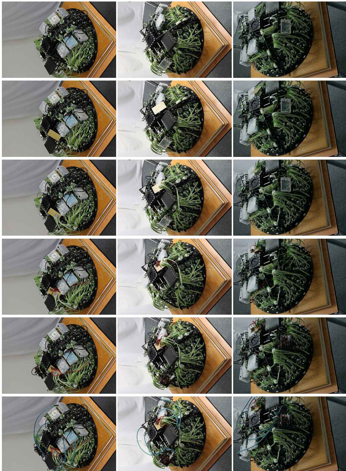
Figure A3. Assembly of lightdrum, step 13 to 18 from three different views. Row 1: mounting the gigabit Ethernet switch and connecting cameras with microcomputers by USB 3.0 cables; Row 2: adding the main RS485 distribution board; Row 3: connecting eight distribution boards to the main one; Row 4: connecting six microcomputers to the power; Row 5: changing the Raspberry Pi 2 cover, adding electronics and connecting stepper motor, laser module and camera for auto-collimator; Row 6: connecting six embedded microcomputers to gigabit Ethernet switch.
