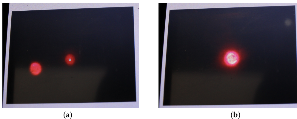
Figure 17. The photograph of the auto-collimator output at the display during operation: (a) the misaligned laser beams giving two spots; (b) aligned (i.e., collimated) laser beams giving one brighter spot.
