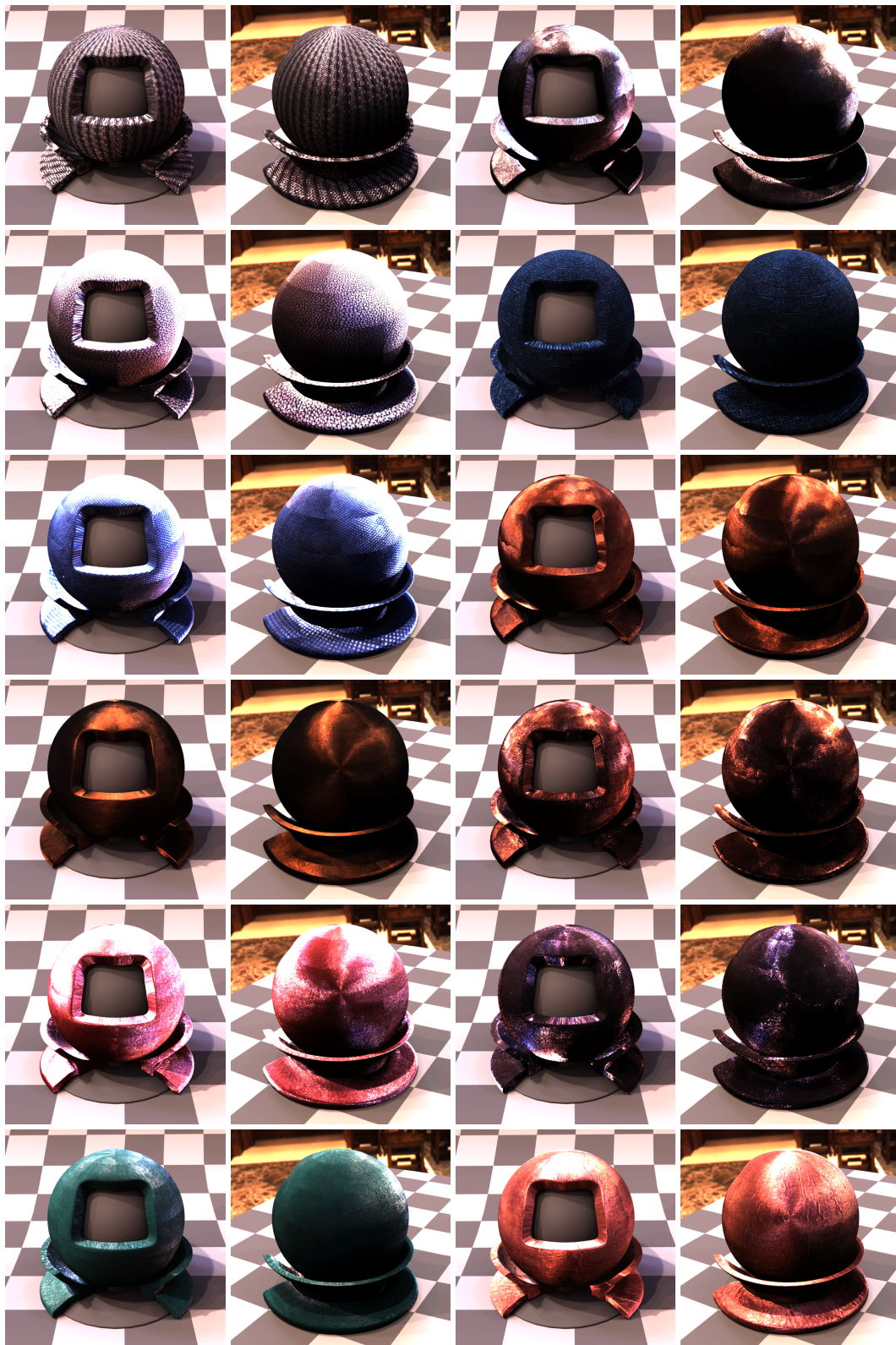
Figure 26. Twelve textile and upholstery material samples, measured by lightdrum, put onto the 3D object and rendered by Mitsuba rendering software under two different views. Materials (top-left to bottom-right): treves2, black leather, tres5, blue denim, fabric003, fabric111, fabric112, fabric135, fabric136, fabric137, fabric300, brocadi001. The materials fabric003, fabric111, fabric112, fabric135, fabric136, fabric137 are courtesy of Jiří Filip.
