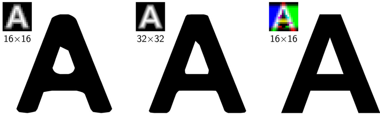
Figure 1: Rendering of the glyph ‘A’ using conventional distance fields at different resolutions ( 16 \times 16 on the left, 32 \times 32 in the middle), and using our multi-channel distance field method at distance field resolution 16 \times 16 (right).
