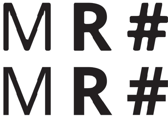
Figure 24: Comparison of the reconstruction of several glyphs of varying thickness using the original (top) and our multi-channel distance field method (bottom).
