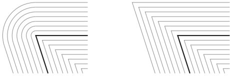
Figure 11: Contour graph of a regular distance field (left) and a pseudo-distance field (right) near a corner.
