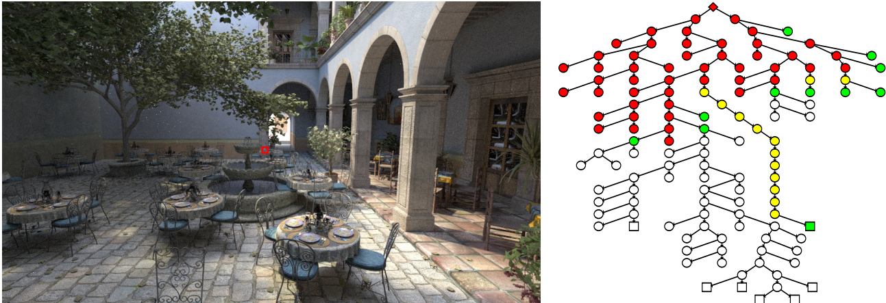
Figure 1: The San Miguel scene and a sample ray corresponding to the central pixel (left), the visualization of tracing the ray using the standard BVH traversal and our method (right). The red nodes are visited only by the standard traversal from the root. The green nodes are entry points of our traversal algorithm. The yellow nodes are visited by neither traversal method and only denote the path to candidate list elements. The white nodes are visited by both types of traversal. In this particular case, our method skips 44% of nodes, both on the path from the BVH root and in lateral branches.
