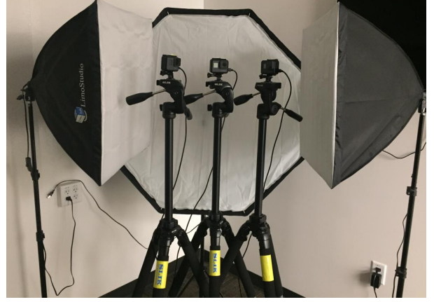
Fig. 3. Our recording setup, featuring three tripod-mounted GoPro cameras and diffuse light sources.
