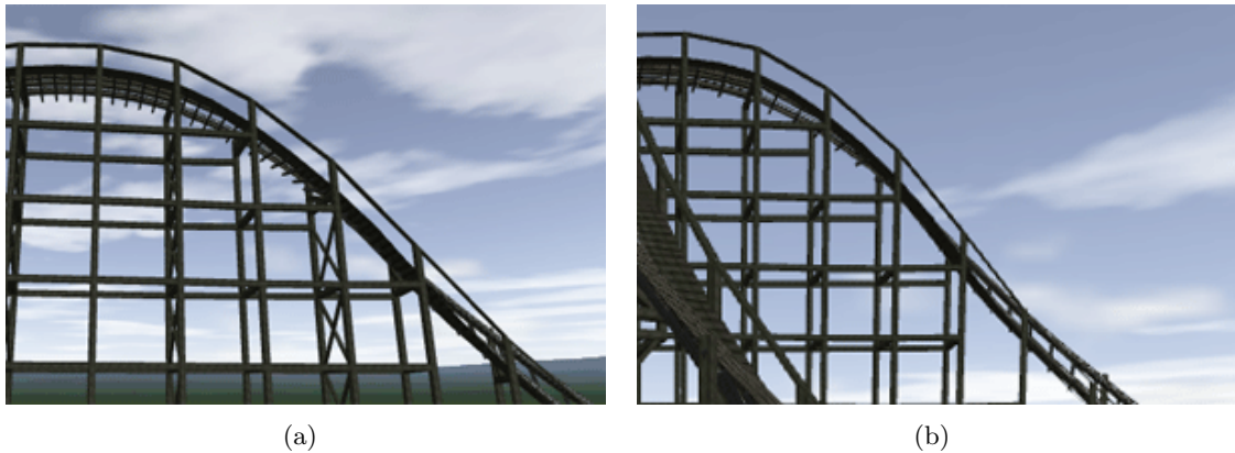
Figure 3.2: Differences between the distance between sleepers and support geometry in different LODs. b) shows the track from bigger distance than a).
