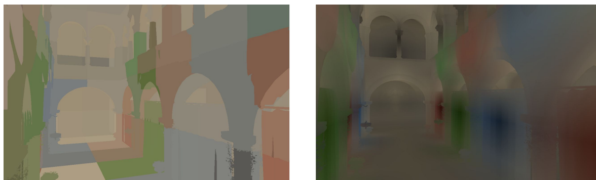
Figure 5.7: The color of the voxel mapped to the surface of the geometry; the color is represented by single value per voxel (on the left); the color of the voxel is represented by brick of 3^3 values (on the right)
