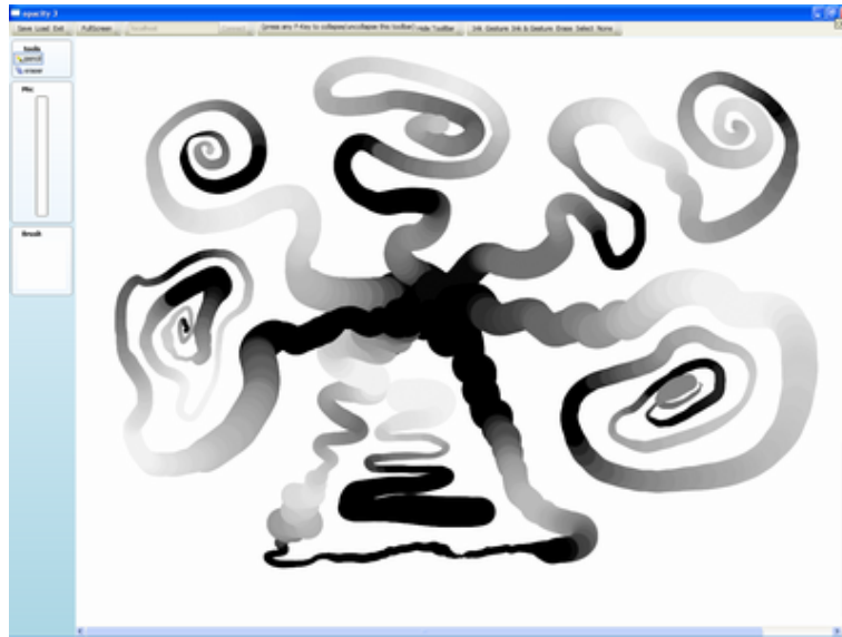
Figure 2.2. Example of a drawing created by using the VoicePen, where the digital stylus was used to specify the stroke thickness and non-speech vocalization was used to specify the opacity [8].
