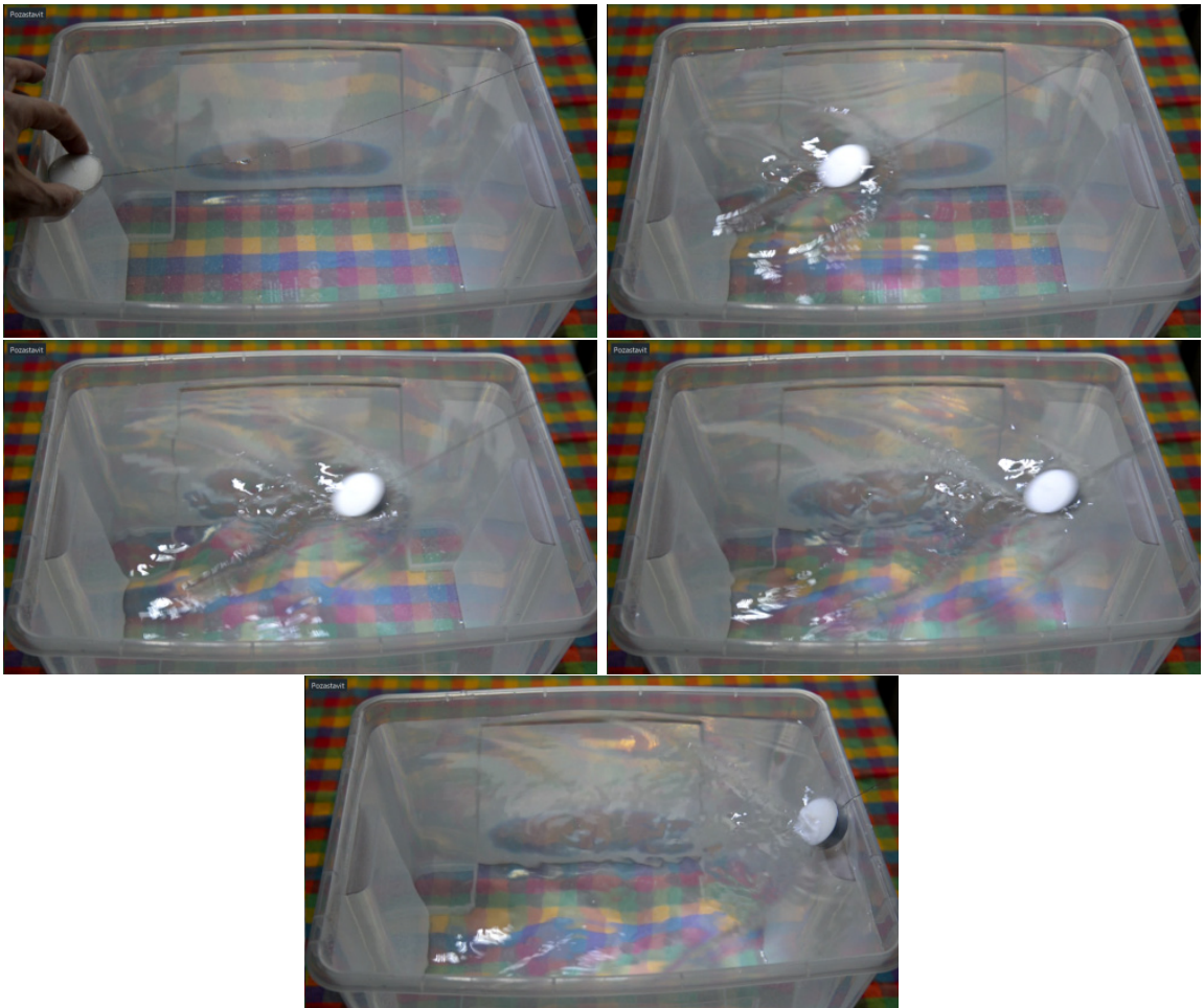
Figure 6.3: Video sequence of real wave propagation in a water tank.
