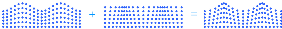
Figure 2.7: Illustration of the horizontal wave. Vertical component (left), horizontal component (centre), compounded wave (right). Courtesy of [YHK07].
