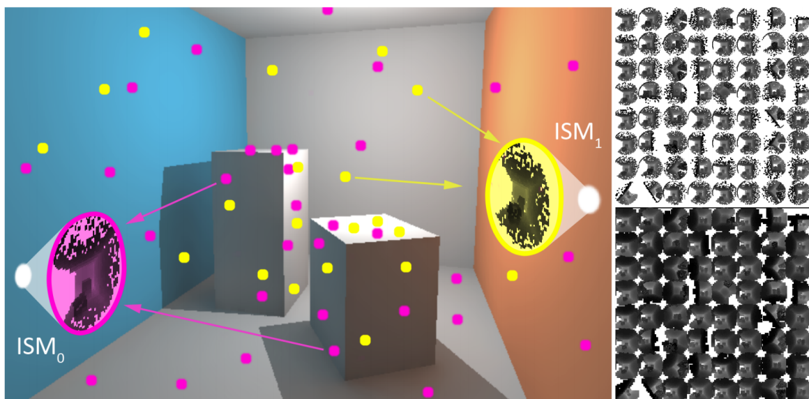
Figure 3.6: Instant radiosity via imperfect shadow maps: A scene point cloud is distributed among the set of VPLs and rendered into an imperfect shadow map atlas (top right). A pull-push algorithm is employed to fill holes present in the shadow maps due to the coarse point representation. Image courtesy of [RGK+08].
