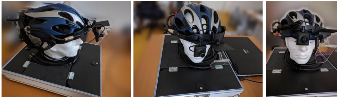
Figure 14 Eye tracking helmet
