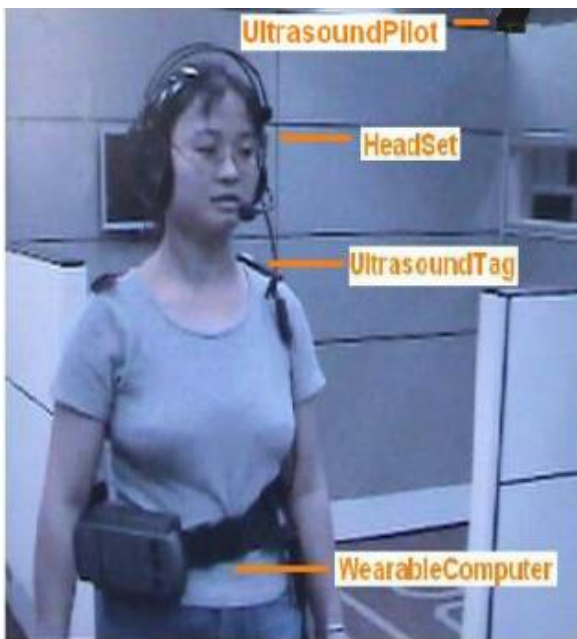
(c) Wearable computer with ultrasound sensors from [64], figure taken from [64]
