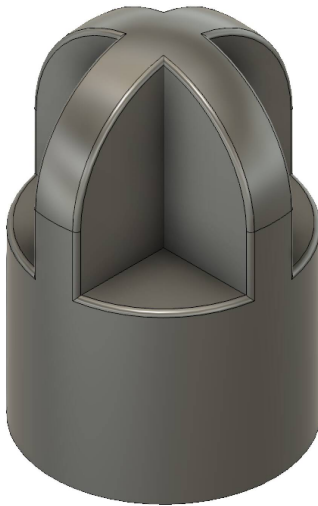
(c) circular knob that represents current location (1cm diameter, 2cm height)
