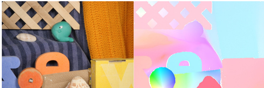
Figure 2.5: An example from the real-life section of the Middlebury dataset [2], acquired by using a special scene with fluorescent paint applied. Image on left represents the camera view and image on the right shows the optical flow field encoded as colors.
