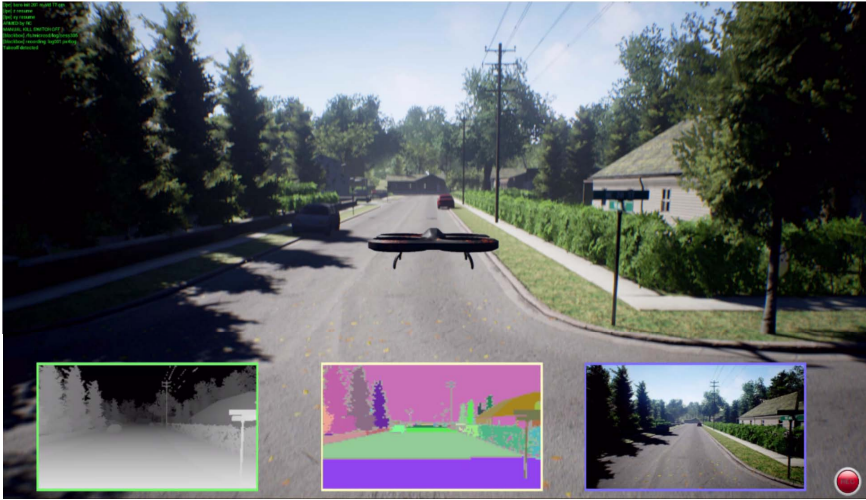
Figure 2.11: A snapshot from AirSim [32] autonomous drone and car simulator, showing different ground truth camera outputs.
