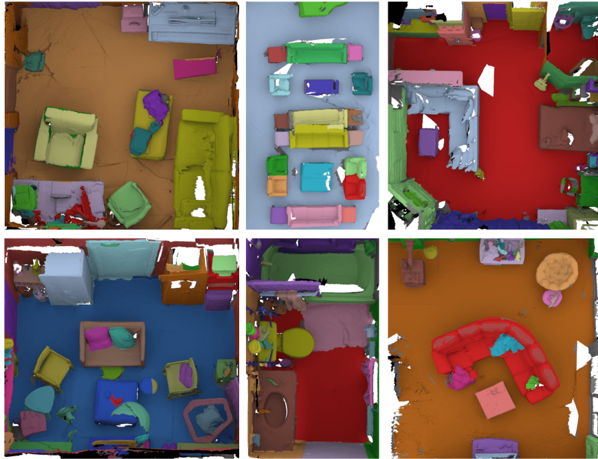
Figure 2.4: The ScanNet dataset [9] was created by using a depth sensor and contains hand annotated 3D semantic segmentation of indoor scenes.
