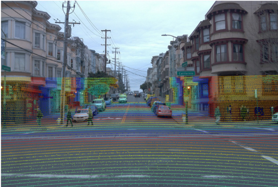
Figure 2.3: An example from the Waymo dataset [33] with the LIDAR data overlaid on top of the image.
