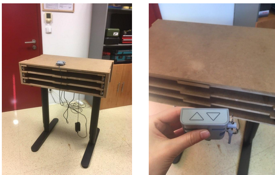
Figure 2.11: First picture: Wooden model of Palata made by Macík following the patent [33]; Second picture: Control to regulate the height of the model.
