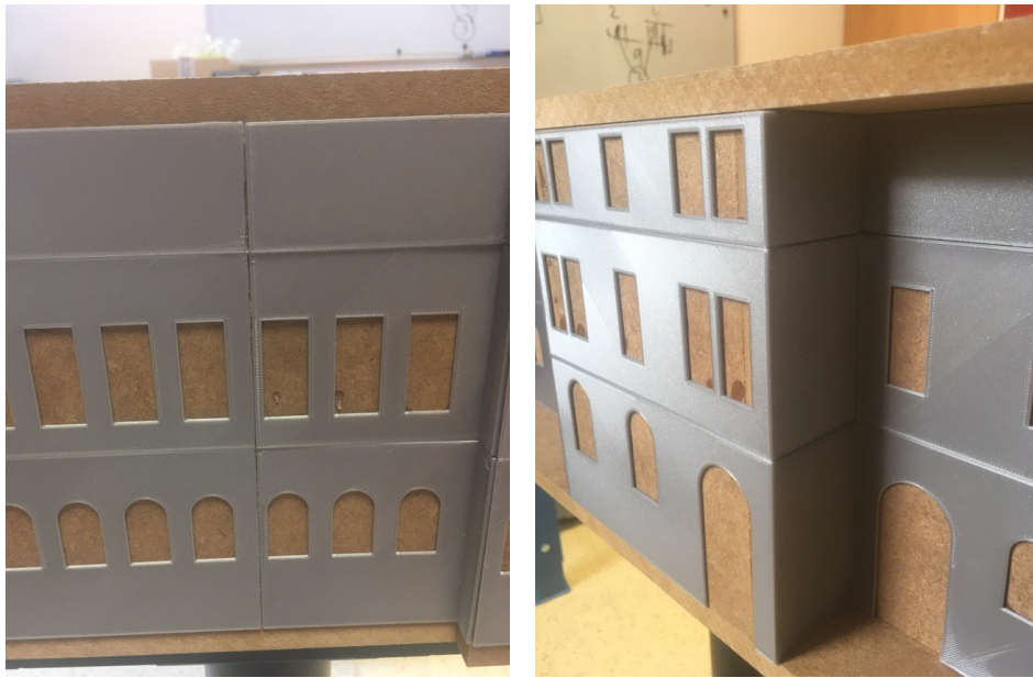
Figure 7.7: First picture: A hole between the tiles. The crossing of four tiles.; Second picture: A "good" corner
