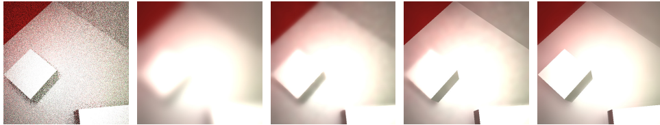
Figure 3.6: EAW with the increasing number of edge weights: unfiltered ray-traced buffer (input), no additional weights: (“pure” À-Trous), ray-traced buffer only (bilateral approx.), two buffers (ray traced, normal) and all three buffers (ray traced, normal, position) (source: [DSHL10]).
