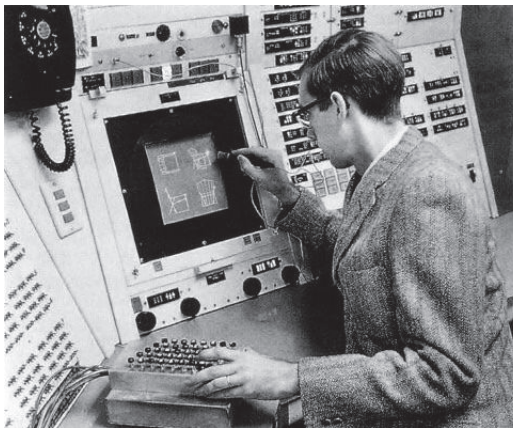
Figure 2.1: (left) Ivan Sutherland using Sketchpad on a Lincoln TX-2 computer in 1963. (right) Utah teapot print on a coffee mug.
