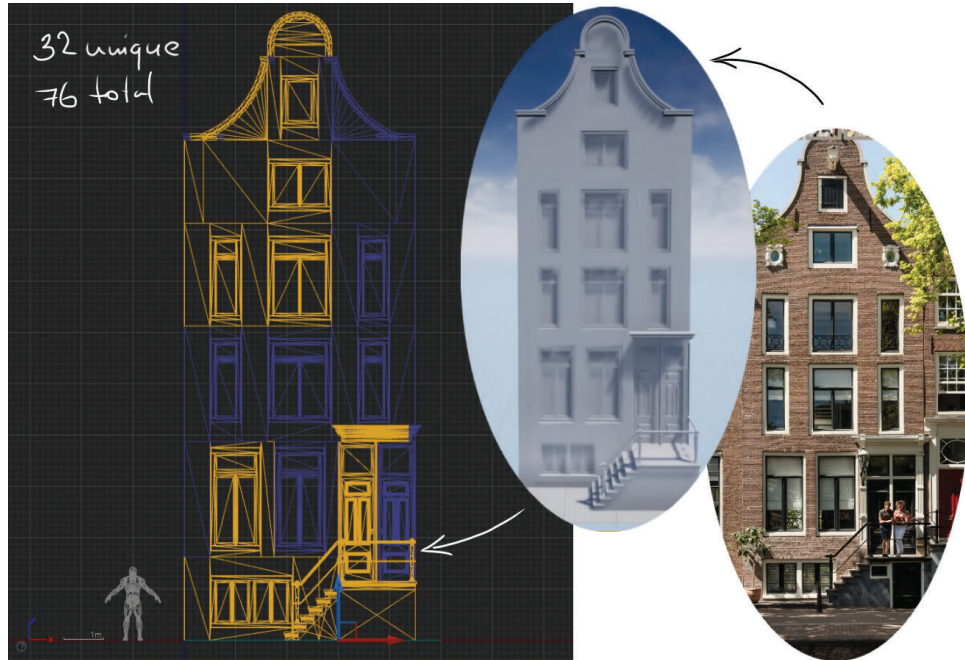
Figure 4.31: (from right to left) A reference image for the building, the final model and its front view representation on the grid inside Unreal Engine. Highlighted in orange are unique assets, while the rest of purple-ish geometry are their instances.
