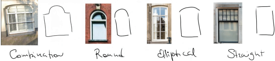
Figure 4.11: Example of each frame head shape
