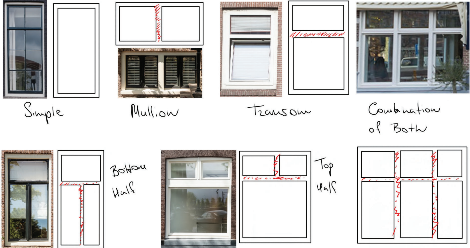
Figure 4.12: Example of each frame type
