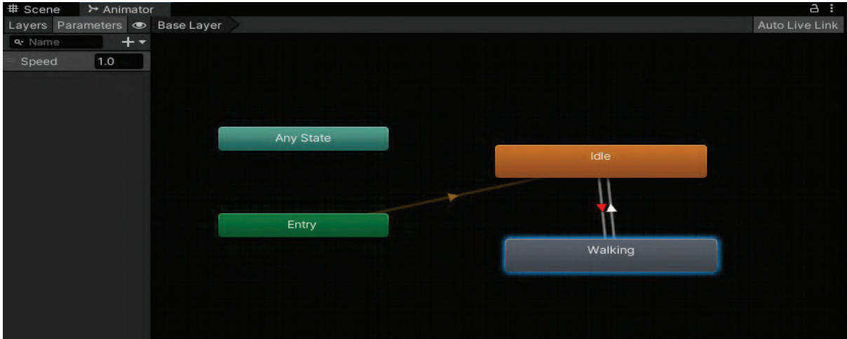
Figure 2.6: the Animator Window with states (Entry, Idle, Walking) and transitions between these states represented by arrows. In the left corner, there is a variable Speed that controls switching of the animations
