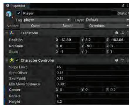
Figure 2.2: The Transform component in the Inspector window with the Character Controller component
