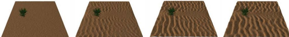
Figure 3.8: Particle based sand simulation with effect of wind shadowing behind vegetation. Captured after 100 s, 200 s and 400 s (from [25]).
