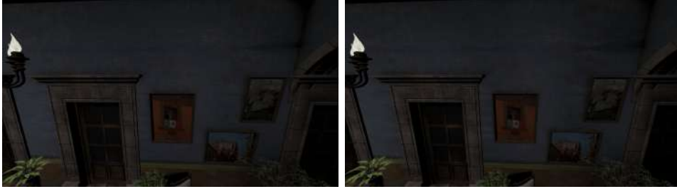
Figure 5.3: On the left image we show the occlusion sampling with the cosine weight and on the right we use wrap diffuse shading. Note that there is no normal biasing. Notice the much more pronounced shadow leaking artifacts next to the door in the wrap shading image.
