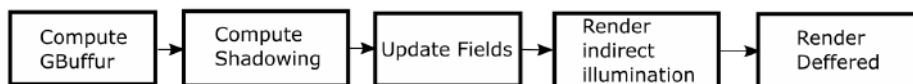
Figure 3.1: A diagram of steps which our renderer takes in each frame to compute the final image.
