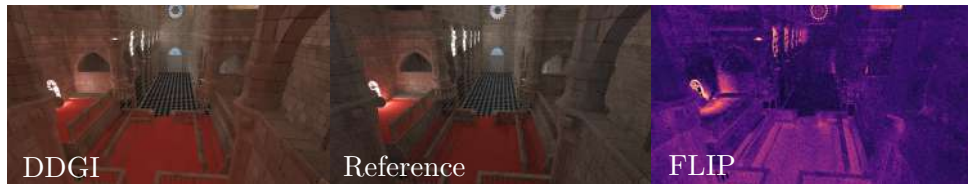
Figure 7.5: Sibenik global illumination comparison. The first Image demonstrates the global illumination produced by DDGI. The next image is our ground truth reference. The last image shows the perceptual image error produced by FLIP. The grid resolution was set to 16 \times 8 \times 12 with 16 \times 16 probe resolution.
