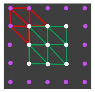
**Figure 3.1:** In this Figure, the green triangles and white points represent the terrain, the purple points are the embalming points used to calculate the normals. The red triangles are all the triangles whose normals contribute to the normal vector of the top left point of the terrain.
