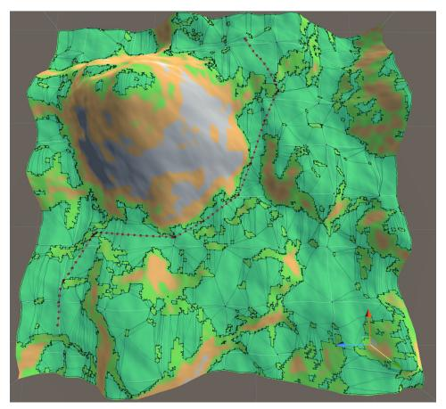
**Figure 3.8:** A straightforward path generated using global path-finding with a NavMesh (turquoise areas). Additionally, for better visibility, the corner points have been connected by more points using linear interpolation.
