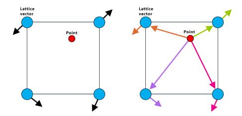
**Figure 2.2:** Algorithm described by subsection 2.1.3. The first picture shows the base setup with lattice vectors and the point at which we want to generate the height. The second picture shows the pairs of vectors that are used for the dot product.
