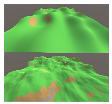
Figure 2.3: Terrain generated with my tool using one octave versus seven octaves.
