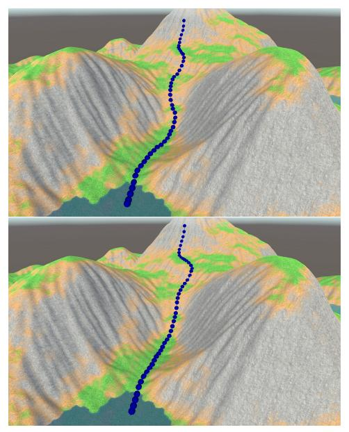
**Figure 3.14:** The first image shows the river agent's path of control points, which follows the gradient more closely than the one in the second image.
