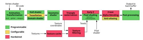
**Figure 3.5:** Modified visualization of the rendering pipeline used in modern applications with color-distinguished stages based on programmability.[12]
