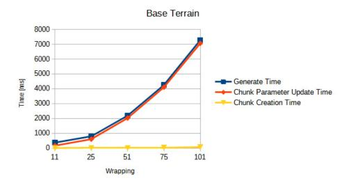
**Figure 4.1:** Graph showing the generation and parameter change times of the base terrain from Table 4.1.
