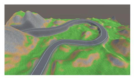
**Figure 3.12:** Terrain with a road generated. The road can heighten the terrain or even cut through it, as seen on the left side of the image.
