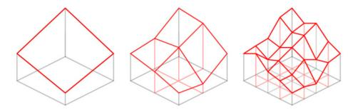
Figure 2.1: Midpoint Displacement algorithm[8].
