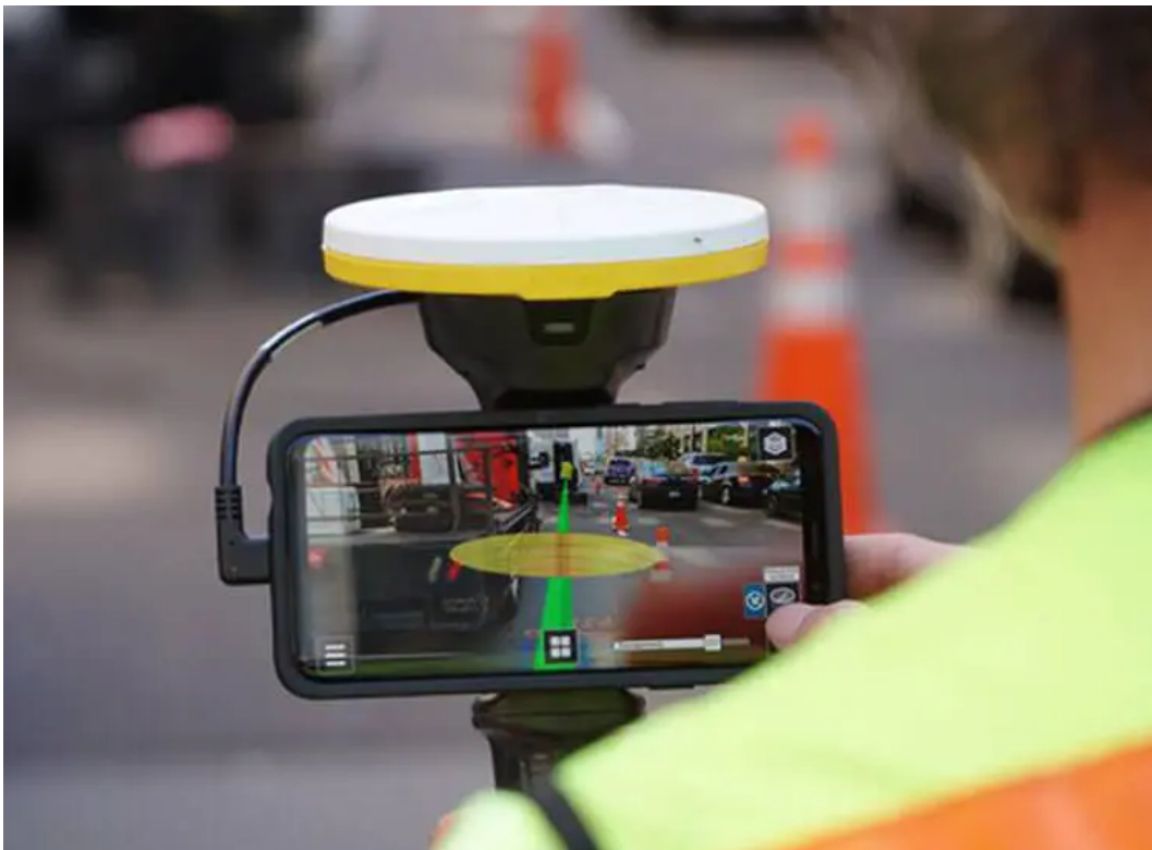
Figure 2.15. SiteVision Positioning system [76].
