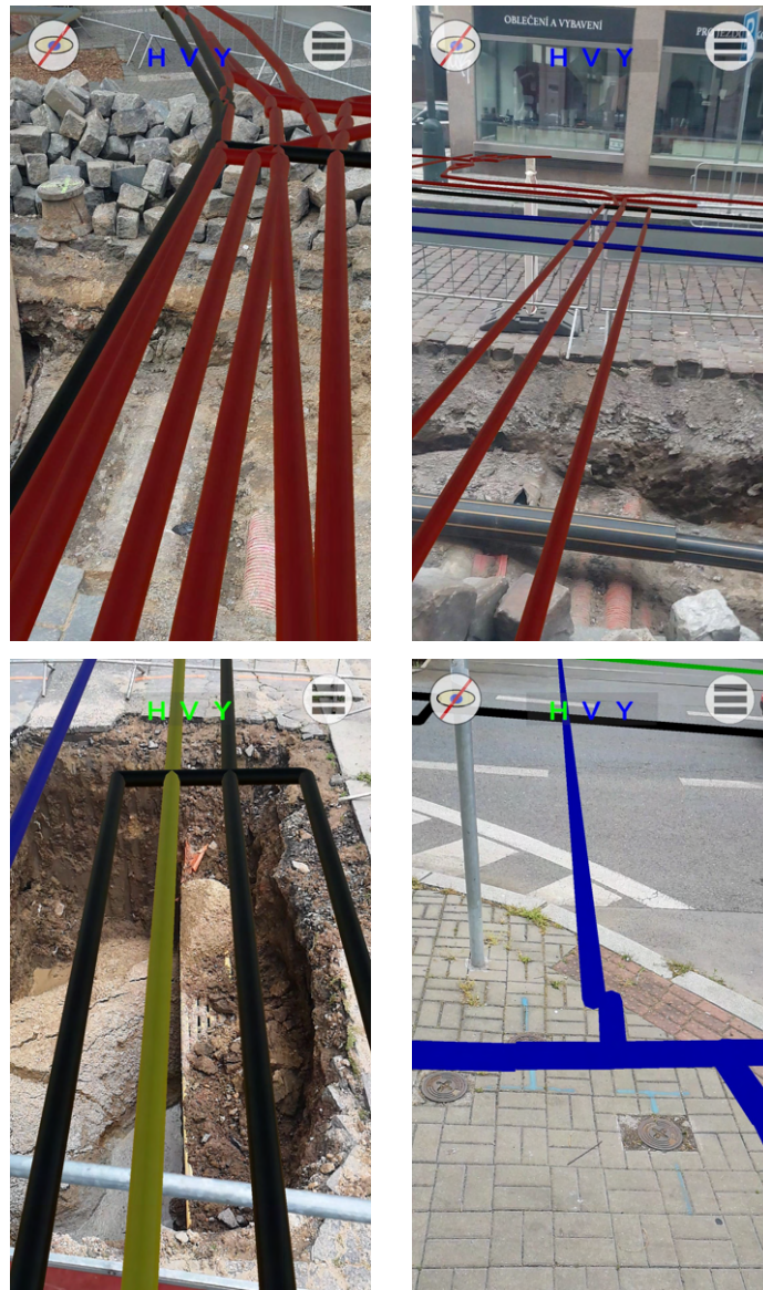
Figure 5.4. Comparison of visualized utility lines with references from the real world.
