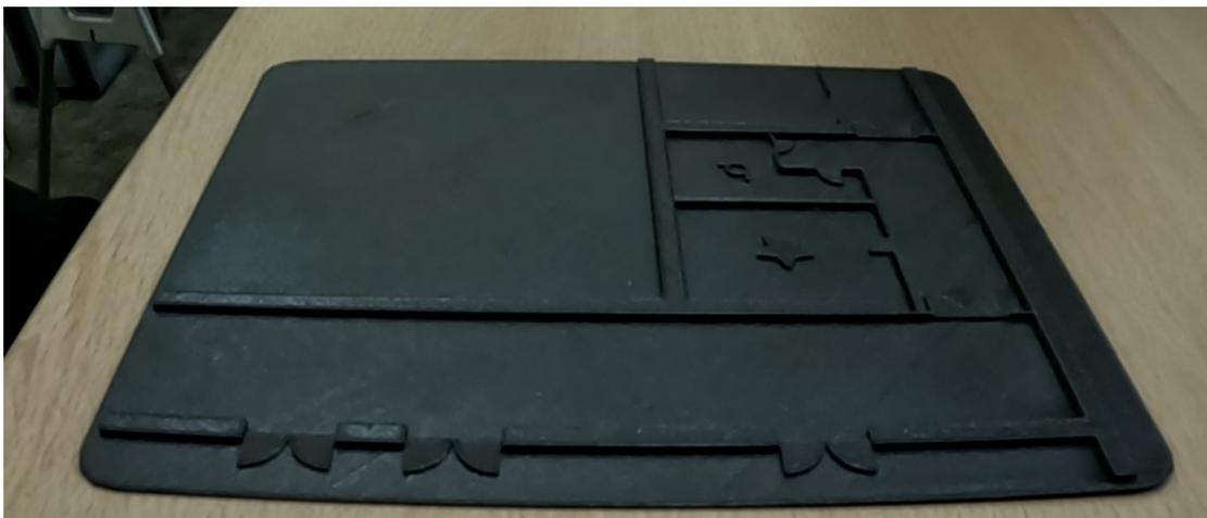
**Figure 6.1.** A tactile map created from the .fbx model of the Unity scene, enhanced by orientation symbols
