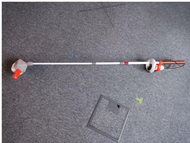
**Figure 5.2.** A photo of the white cane including the physical brake
