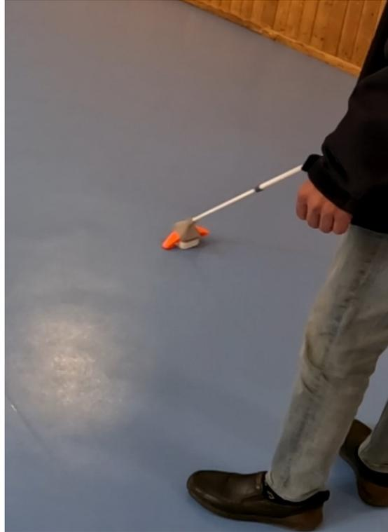
**Figure 6.2.** The cane tip can be quite easily tilted when in fast motion and even the slightest angling of the tip can lead to the haptic feedback not being perceivable.
