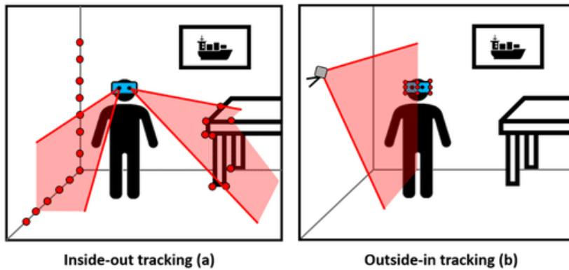
**Figure 2.3:** Illustration of inside-out (a) vs. outside-in (b) optical tracking[29]
