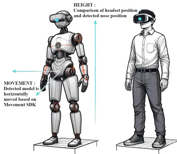
**Figure 3.4:** Sketch of the continuous position and movement calculation
