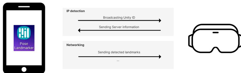
**Figure 3.2:** Scheme of the UDP communication between the MediaPipe Android application and the VR prototype
