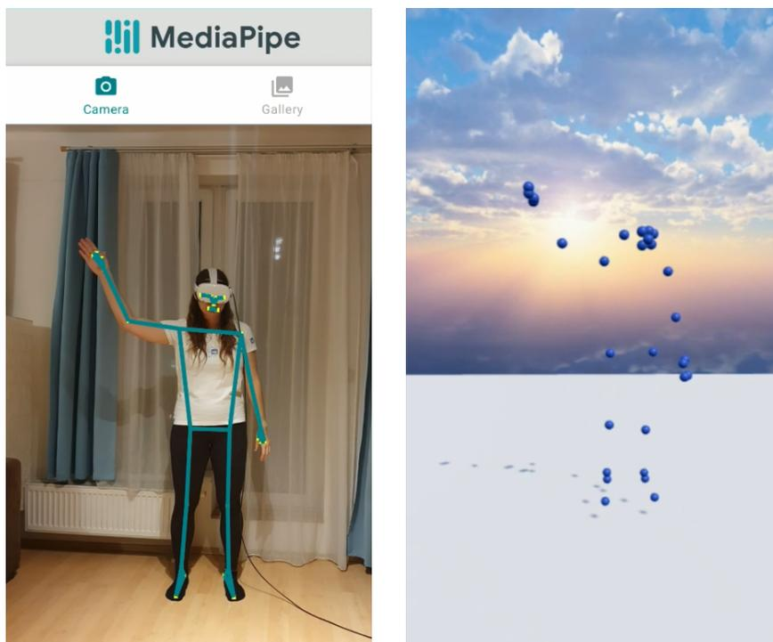
**Figure 3.3:** Landmarks detected in the MediaPipe application (*on the left*) and their initial representation in the virtual environment (*on the right*)
