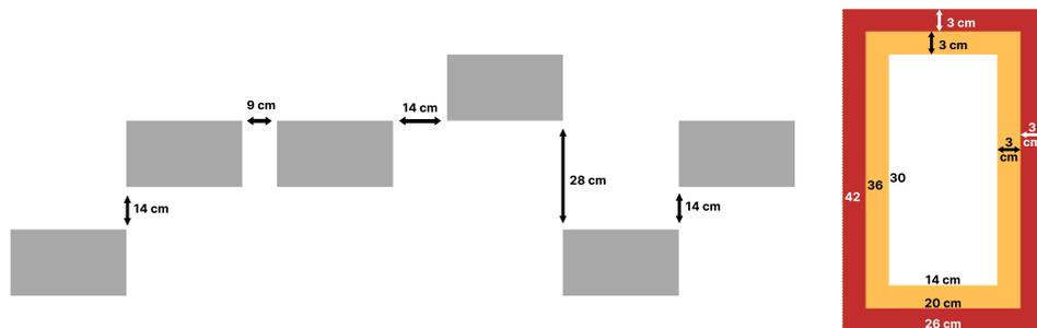
**Figure 4.1:** Schema of the optimal test path (*on the left*) and the enlarged testing step area with three regions used for accuracy measurement (*on the right*)
