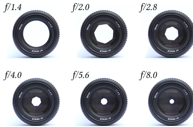
Figure 2.3: Iris aperture with changing f-number, image taken from [4]
