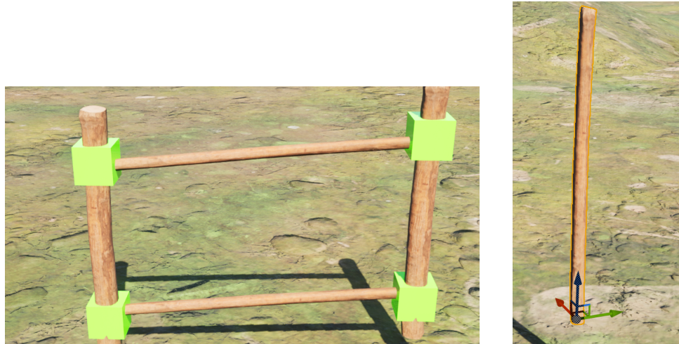
(a) : Rails correctly spanning between sockets on adjacent posts.
