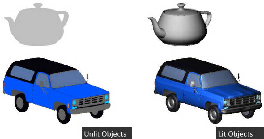
Figure 2.3: A comparison of the same objects rendered with material color only (left) and with both color and shading (right). Notice the lack of depth in the first image (source: [FS22]).
