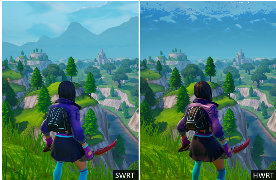
Figure 5.30: A visual comparison of Fortnite’s outdoor scenery when using software (SWRT) and hardware ray tracing (HWRT). Notice the lack of direct shadowing on the player character and the missing storm when using SWRT. Rendered on PC 2 using the Lumen Epic configuration.
