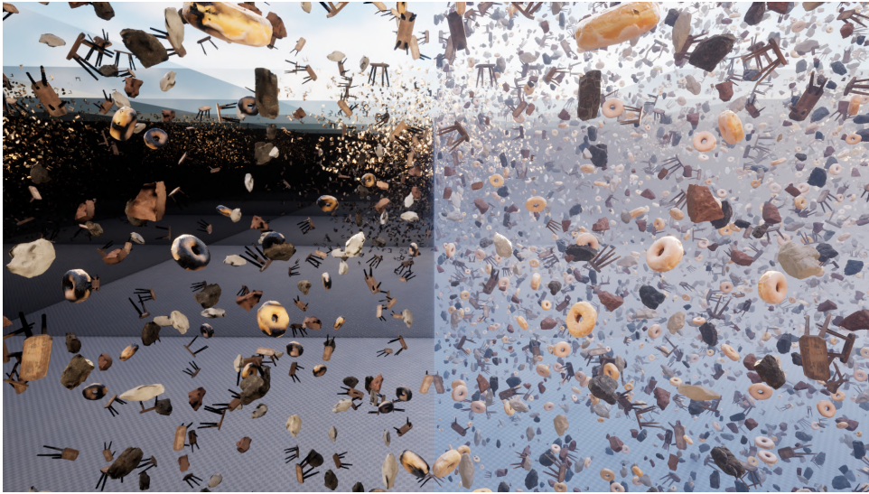
Figure 5.27: A screenshot of the Performance Testing scene with 18 000 objects. Notice how the majority of objects does not appear in the mirror reflection on left. Furthermore, some of those which do appear have missing surface cache coverage, thus partially showing as black. This image was rendered using hardware ray tracing with Lumen High, Nanite and the Hit-Lighting pipeline.
