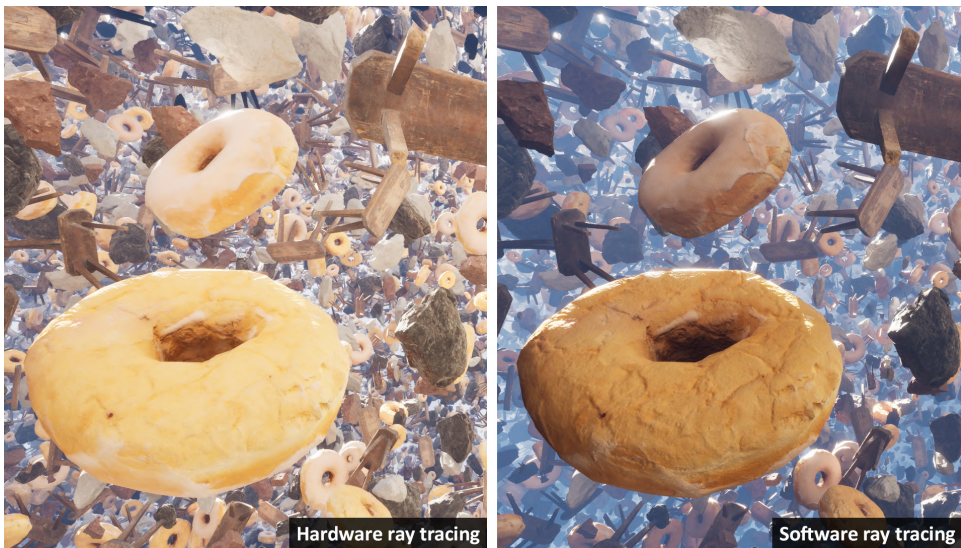
Figure 5.28: A visual comparison between hardware and software ray tracing. Rendered with Nanite and Lumen Default.
