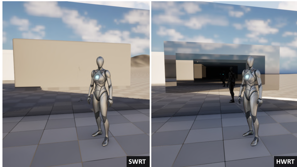
Figure 5.12: A comparison of multi-bounce mirror reflections rendered using Lumen High on software and hardware ray tracing on PC 1. Notice the black character and downsampled skybox in reflections.
