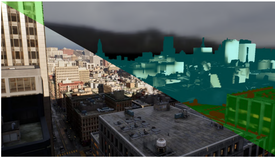
Figure 4.11: A visualization of the different scene representations used in HW ray tracing. Near-field is shown in green, far-field in cyan, and the brown areas have missing surface cache coverage (source: [WNK]).
