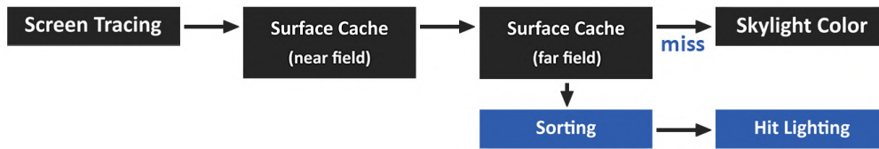
Figure 4.9: A scheme of Lumen’s ray tracing when using hardware ray tracing. The steps highlighted in blue are performed only when using the hit-lighting pipeline.
