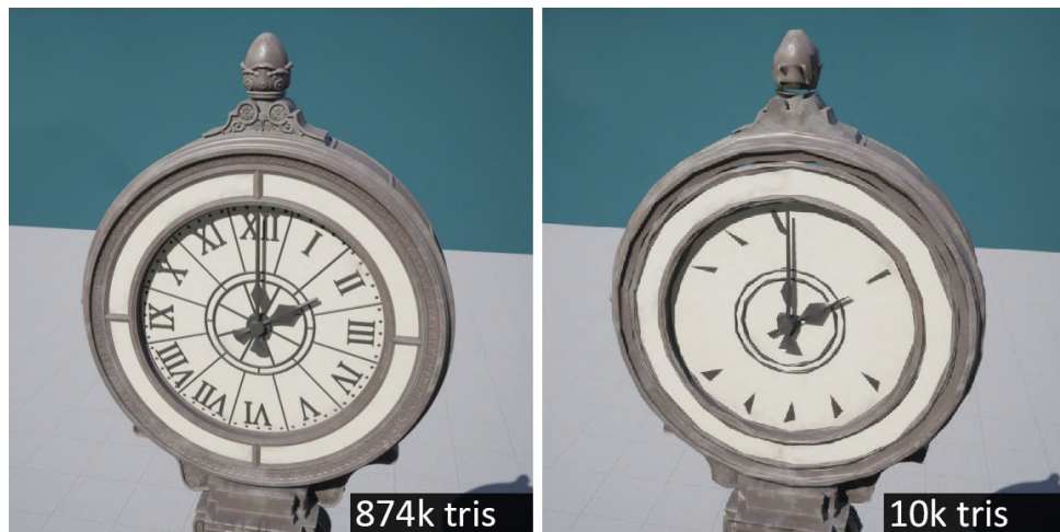
Figure 4.3: An illustration of a difference between a (on the left side) and its fallback variant (on the right side) used for hardware ray tracing, along with the corresponding triangle counts (source: [WNK]).
