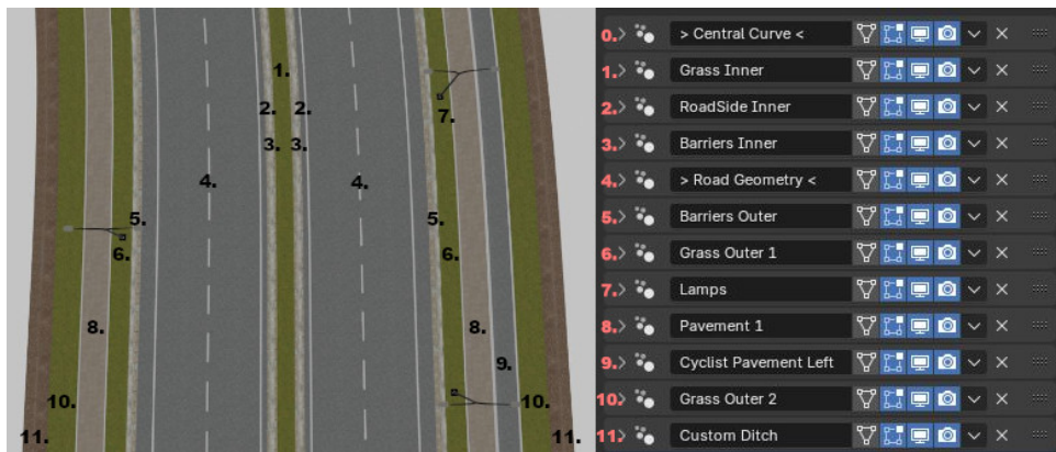
Figure 8.2: Demo of road features generated geometry and corresponding modifier stack
