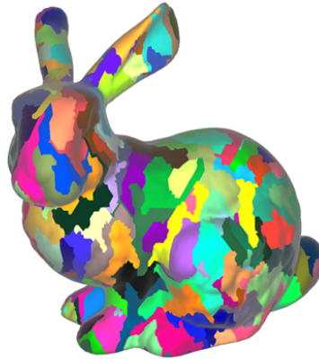
Figure 3.2: Mesh split into meshlets [31]
