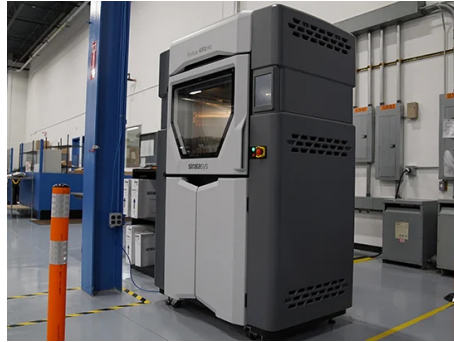
Figure 2.5. Industrial 3D printer Fortus 450mc. Image taken from [7].
