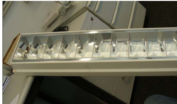
Figure 9.19: Holder and cover for luminaire # 3.
