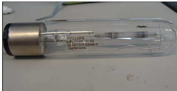
Figure 9.35: Gaseous discharge lamp of luminaire # 5.
