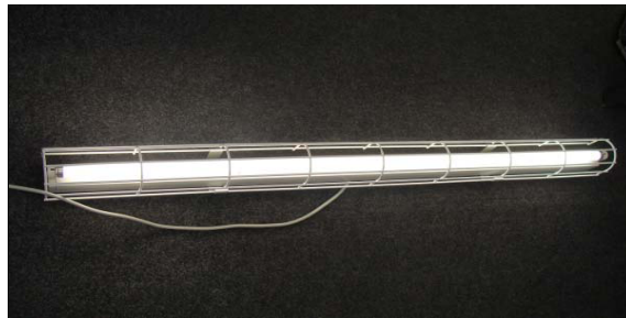
Figure 9.10: Luminaire #2 without light shield switched on.
